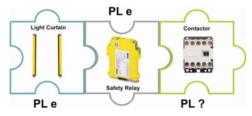
Figure 1. Safety circuit rated for Performance Level "c"
